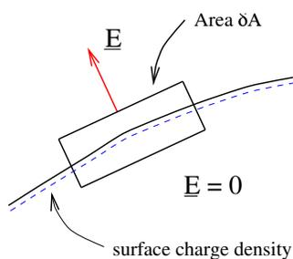
Consider applying Gauss' Law to the infinitesimal “pill-box” of height  $\delta h$  and area  $\delta A$ , as shown. Within the conductor,  $\mathbf{E} = 0$ , and at the surface of the conductor  $\mathbf{E}$  is *normal* to the surface.
